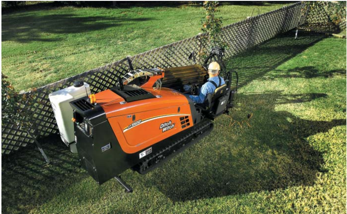
When a fence or other constraints challenge drilling for GSHP loops the Ditch Witch 922, a machine the size of a small garden tractor, could provide an answer. (Photo courtesy of Ditch Witch.)
